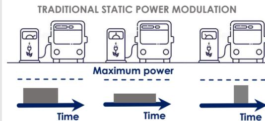
MaeStor is able to perform an optimized **dynamic modulation** of the charging power for each vehicle in the fleet according to the specific efficiency characteristics of the battery/charger set.
