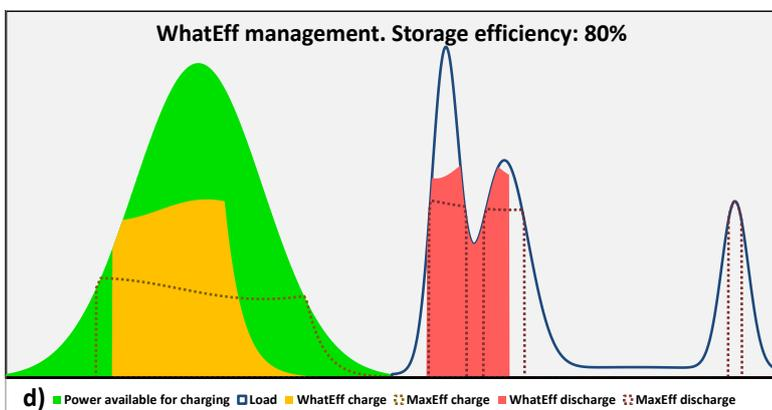
Fig. 4. Example of NomoStor application: 4a) typical profiles of power available for charging and loads; 4b) traditional storage management; 4c) storage management according to NomoStor MaxEff operating mode; 4d) storage management according to NomoStor WhatEff
