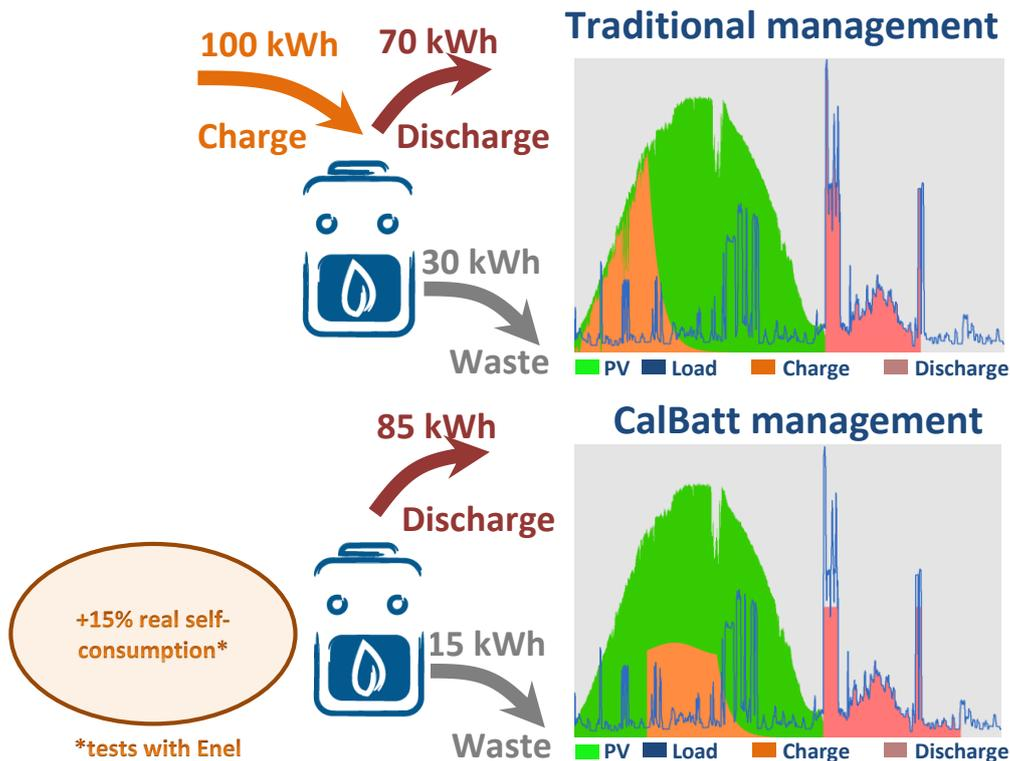
**Fig. 1: conceptual example showing the difference between the conventional and the innovative CalBatt approaches to energy storage management**
