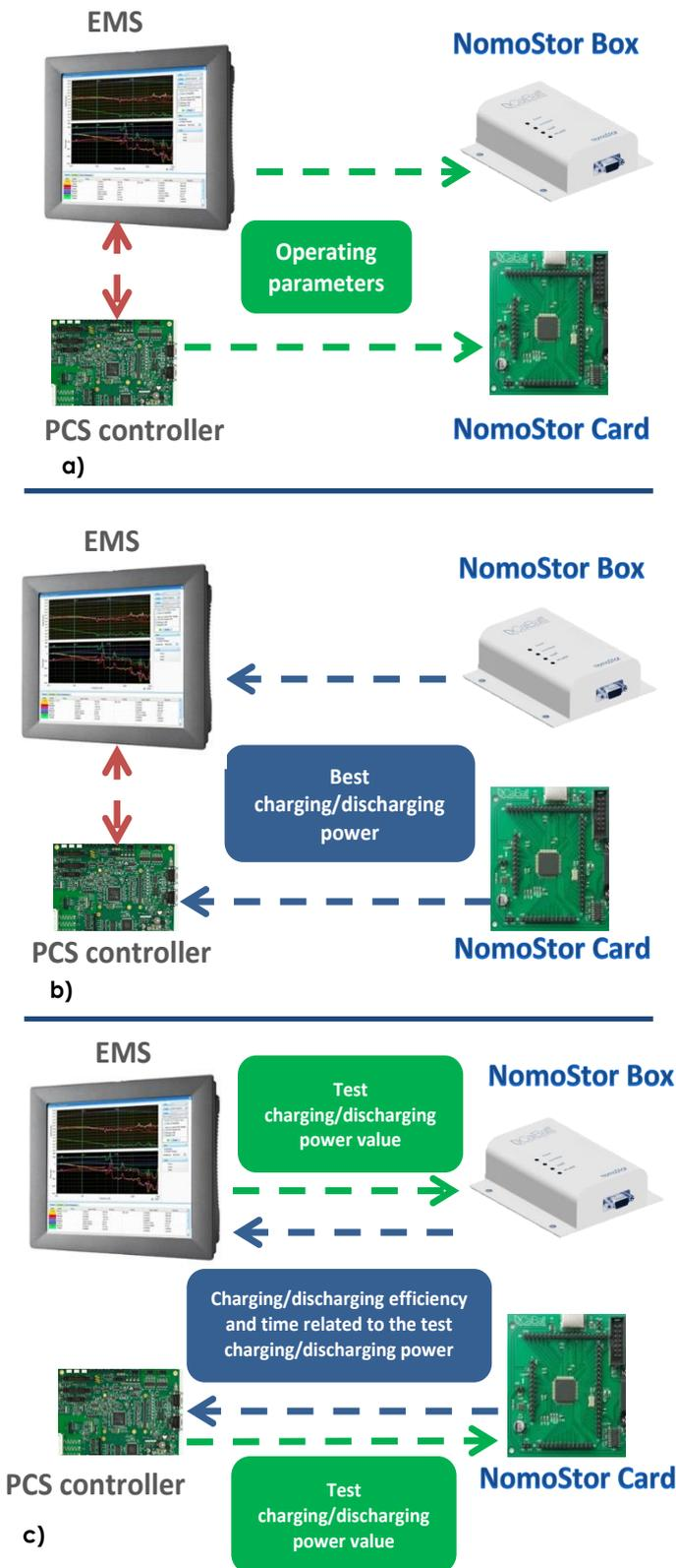
**Fig. 3. NomoStor interaction with the other blocks of the storage system in the three different operating modes available: 3a) DynAnalysis mode; 3b) MaxEff mode; 3c) WhatEff mode.**
