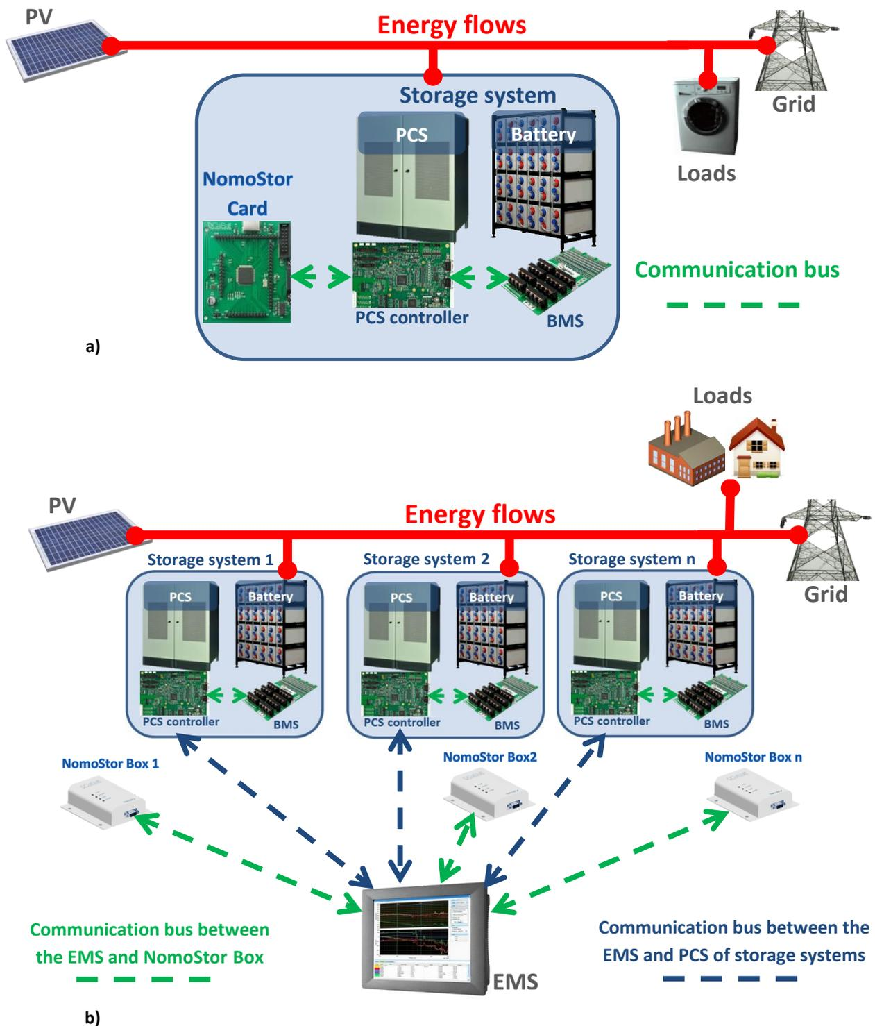
Fig. 2: block diagram showing the connection of CalBatt NomoStor with the devices of the storage system: 2a) NomoStor Card embedded into the storage system and interacting with the PCS controller; 2b) NomoStor Box as a stand-alone device interacting with the EMS external to storage systems.
